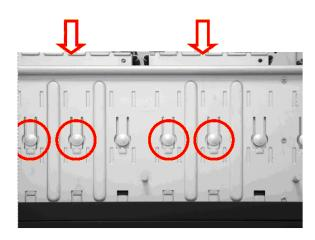
First press the two round shape button using your thumbs, then use your index finger to push the 3.5" module to remove it.
